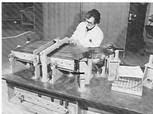
Fig. 16 - Steel wing attachment fittings accurately mounted in welding fixture.
