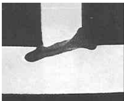
Fig. 28 - Laser welded T joint in 3.2 mm thick plate.
