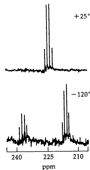
FIGURE 7.32. Carbon-13 NMR spectra of the B isomer of \text{Cp}_3\text{Rh}_3(\text{CO})_3 at room temperature and at -125^\circ\text{C} . [Reprinted with permission from R. J. Lawson and J. R. Shapley, Inorg. Chem. 17, 772 (1978). Copyright 1978 American Chemical Society.]
