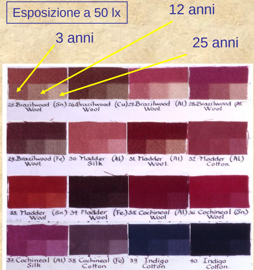
FIG. 1. Some of the faded specimens. The rectangular areas are unexposed. The three square areas on each specimen have been exposed to 7.8, 36 and 91 million lux hours of light from Atlas "Northlight" fluorescent tubes. In all the dycings illustrated here the palest area has received the greatest light dose. The GS difference between exposed and unexposed dye is written on the unexposed part.
