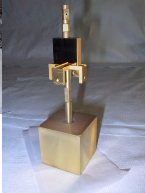
Hollow proof-mass for torsion pendulum testing
