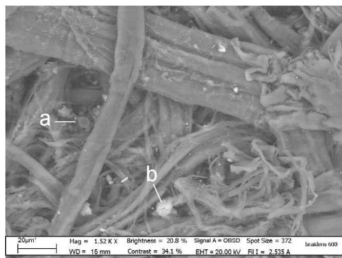
Fig. 7. Scanning electron micrograph of an uncoated sample. The image was obtained with a backscattered electron detector (QBSD). The differences in average atomic number of the organic and inorganic materials allowed for well-contrasted observation of filling materials and ion distribution on paper surfaces. Cellulose fibres of different sizes and with different degrees of integrity can be examined with detail in SEM pictures; fungal spore (a), crystals and aggregates of sizing materials and of impurities (b) are also visible.
